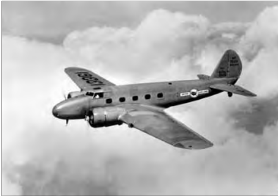
The Boeing 247D integrated all the most desirable features emerging from the airplane design revolution, making it the first “modern airliner.” (SI Negative No. 75-12118)
