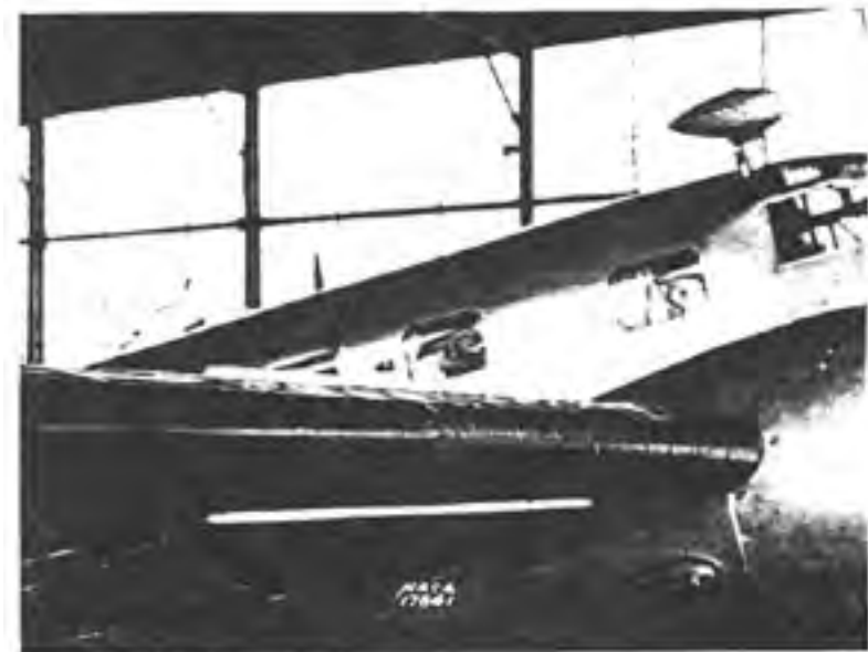
Figure 8.- Rubber de-icer with simulated ice only on cap strips. Drag condition (4).
