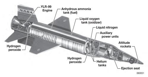
This cutaway drawing reveals the volume of tankage needed to give the X-15 its dazzling propulsion, its pressurization, and its attitude control in space. Liquid-oxygen capacity, 1003 gal.; anhydrous-ammonia capacity, 1445 gal.
