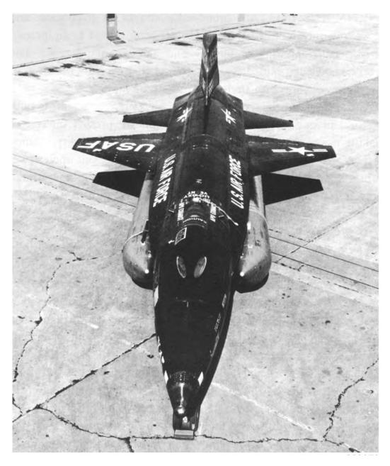
Here's the X-15-2 (rebuilt following the McKay accident) with jettisonable fuel tanks attached to its side fairings. Those tanks carry an extra 13 500 lb. of propellants and will boost the plane's top speed to Mach 8 or provide longer flights. The plane's surface must be covered with an ablative coating to protect its structure from the 4000-deg. air temperatures of Mach 8 flight.
