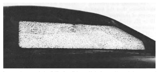
A noteworthy scar of the X-15's first flight to Mach 6 was this cracked outer panel on the right side of the windshield. Investigators found that thermal stresses higher than expected in the metal retainer holding the glass had caused the cracking.
