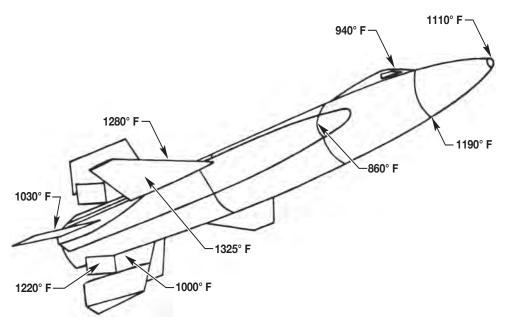
research contribution of Consequently, the the X-15 has been through clearer aerodynamic heating understanding of heat transfer and local flow conditions across a turbulent boundary layer. This pioneering work showed initially that heat flow into the X-15 was 30-40 percent lower than predicted by available theodiscrepancy, while favorable to keeping ries. This large temperatures low during flight to high speed, stimulated further analysis of the flow conditions.
