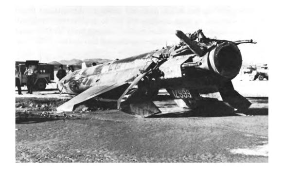
One such landing resulted in abnormally high loads because of a heavyweight condition from incomplete jettisoning of all unused propellants, and only partial cushioning of the nose impact by the nose-gear shock strut. When the nose wheels touched down, the fuselage buckled just aft of the cockpit, causing it to drag on the ground. Fortunately, the damage was easily repaired, and the airplane was back in the air within three months.
