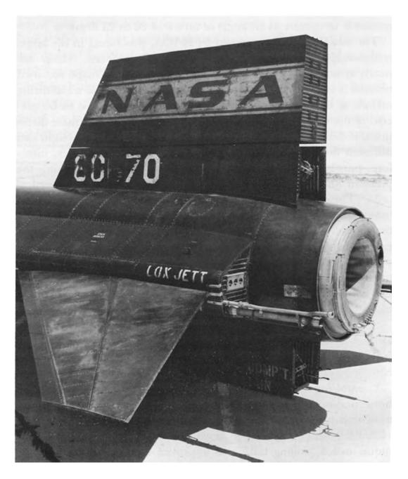
The blunt aft ends of the X-15's side fairings, vertical tails, and the rocket-engine nozzle represent one of the many compromises that a hypersonic configuration demanded. Together they produce as much drag as an F-104 jet fighter.
