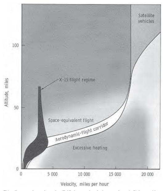
This diagram shows how the X-15 has explored the aerodynamic-flight corridor to a speed of 4000 mph and the space-equivalent region above it to an altitude of 67 miles. The aerodynamic-flight corridor is the pathway that reentry spacecraft of the lifting-body type would use to return to Earth from orbital space stations.
