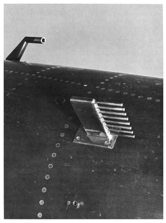
One of the many tools of the X-15's research is this multiple-probe pressure take, mounted on the forward fuselage to measure boundary-layer airflow at hypersonic speeds. Below the rake is one of the 140 holes cut in the aircraft's skin to measure surface pressures. Above and behind the rake is a pressure probe, used only during landing, for the pilot's airspeed indicator.
