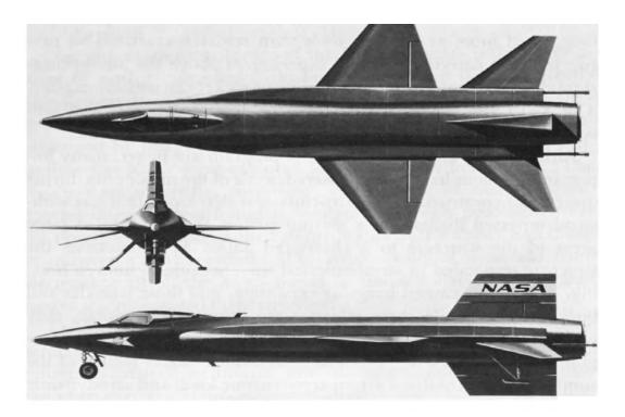
Three views of the X-15's original configuration, with which it achieved a maximum speed of Mach 6.06 and a maximum altitude of 354 200 ft. Its launch weight was 33 000 lb.; landing weight, 14 700 lb. The lower half of its vertical tail had to be jettisoned before landing, since, as the little head-on view makes clear, it otherwise would have protruded below the landing gear when the latter was extended.
