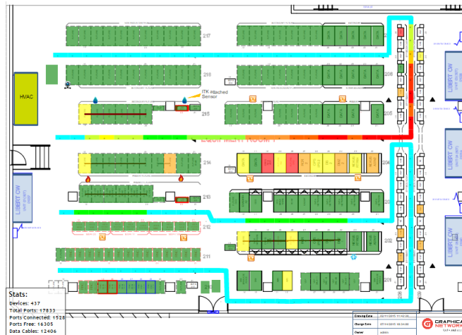
Figure 6. An example display for how server temperature and power information can be used to monitor the state and performance of a DC [47].
