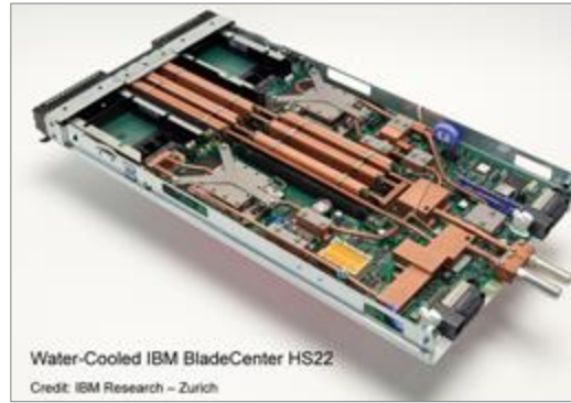
Figure 29. Example of a modified blade server with the hardware required for direct-to-chip cooling [148].
