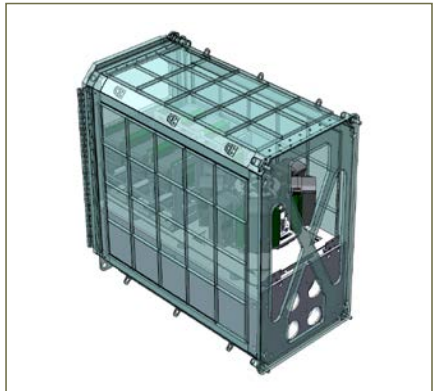
Figure 8: NanoRacks Platform 3 assembly for insertion in an EXPRESS Rack.
