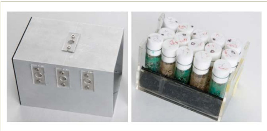
Figure 12: HEART Flies NanoRacks container (left) and the 15 vial assembly ready for insertion.
