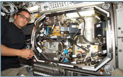
Figure 9: Zero Boil-Off Tank (ZBOT) hardware in the Microgravity Science Glovebox (MSG) aboard ISS with Astronaut Joe Acaba.
