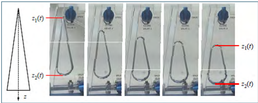
Figure 15. Image sequence of Interior Corner Flow2 bubble migration where each image is approximately 60 seconds apart. The bubble location measurements, z_1 and z_2 , are tracked and compared with analytic and numeric predictions.
