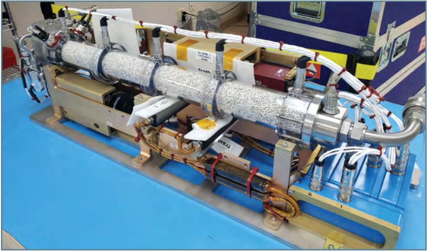
Figure 11: Packed Bed Reactor Experiment (PBRE) Test Section and Diagnostics.
