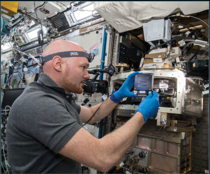
European Space Agency astronaut Commander Alex Gerst conducts operations to reconfigure the Light Microscopy Module (LMM) from Advanced Colloids Experiment-Temperature-7 (ACE-T-7) experiment operations to Biophysics experiment operations. He is holding a removed ACE Module. (Image credit: NASA)
