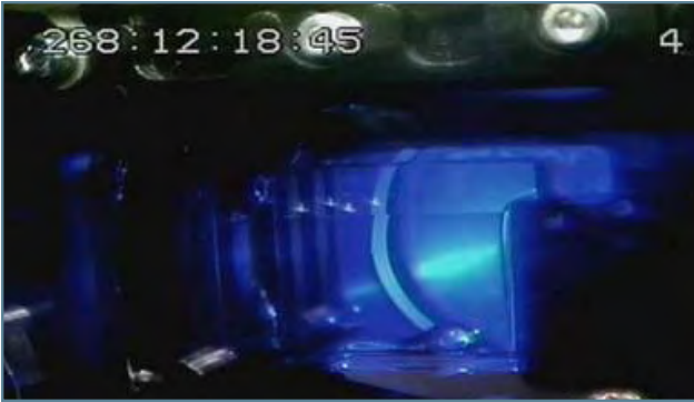
Figure 19. Capillary Channel Flow image of Experimental Unit #2 using second Microgravity Science Glovebox camera. The bubble in lower portion of image indicates the critical flow rate has been reached for this test point.
