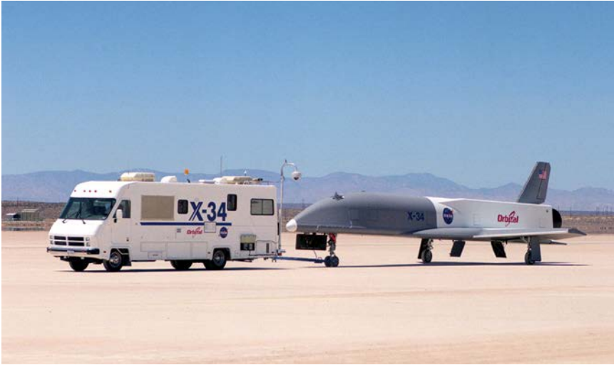
The Orbital mission operations vehicle (MOV) shown with the X-34 A-1 during ground navigation trials at the NASA Dryden Flight Research Center, July 20, 2000. (NASA)
