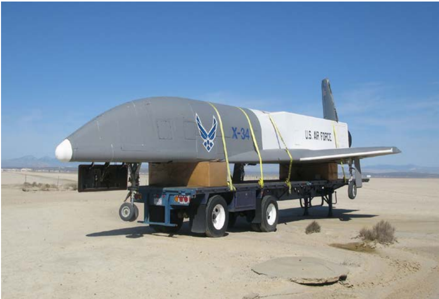
The X-34 A-1A is sitting on a flatbed trailer on the east lakeshore of Rogers Dry Lake on March 17, 2010. Notice that the canted vertical fin has been damaged by the gusting desert winds. (RPH)
