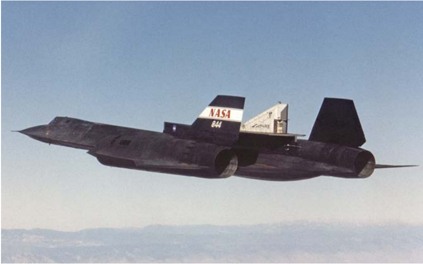
A Dryden Flight Research Center Lockheed SR-71A Blackbird flew with a special linear aerospike experiment (LASRE), although it only achieved “cold” non-ignition flow. (NASA)
