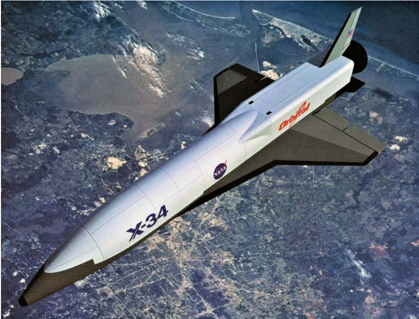
This is an artistic conception of the Orbital X-34 Technology Testbed Demonstrator during a Mach 8 hypersonic glide. (NASA)
