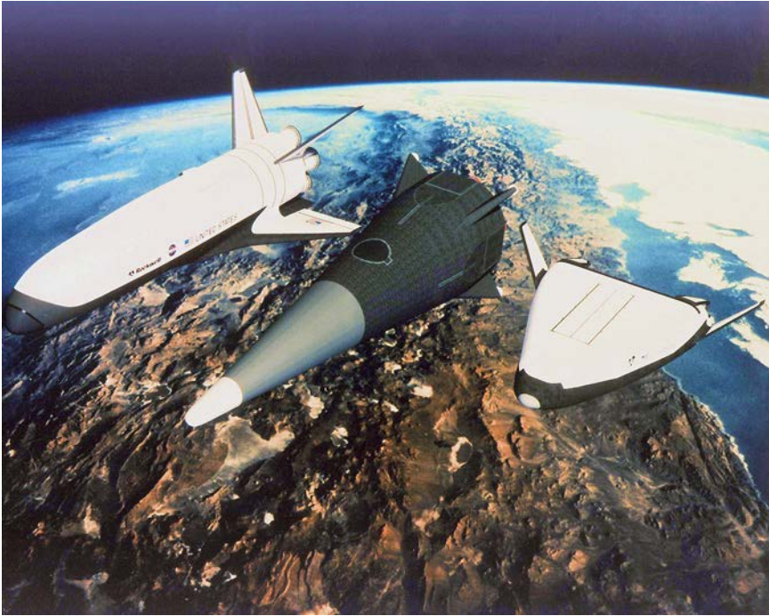
These were the three candidates for the X-33 Phase I design concepts from 1995. They are (L to R) the Rockwell winged RLV, the McDonnell Douglas-Boeing VTO/VL RLV, and the Lockheed Martin lifting body RLV. (NASA)
