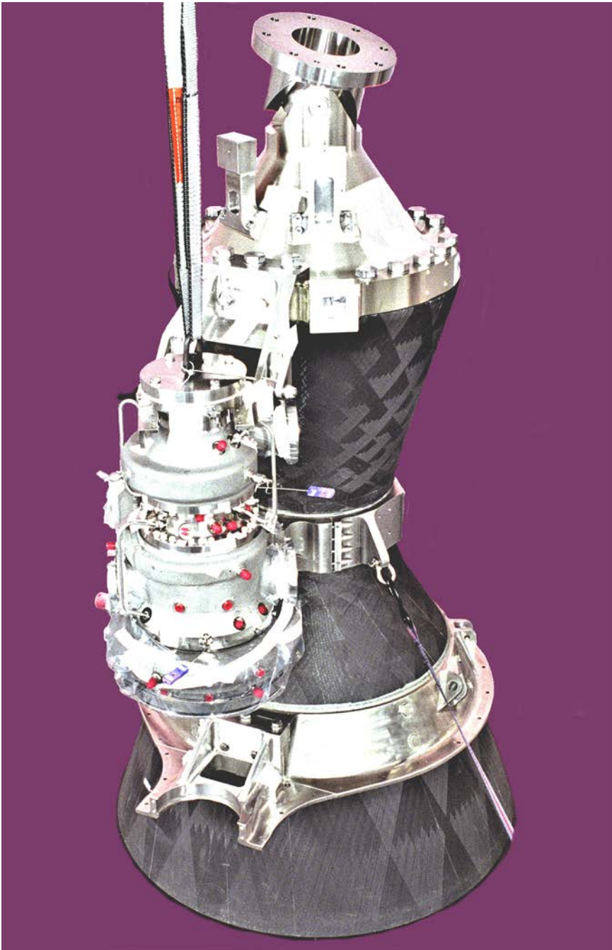
The NASA MC-1 Fastrac 60,000 pound-thrust liquid fuel rocket engine was intended for the X-34 research vehicle. (NASA)
