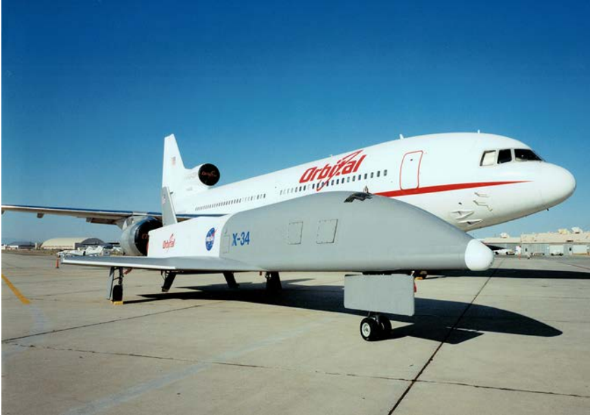
The X-34 A-1 with its Lockheed L-1011 mother ship, on the ramp of the NASA Hugh L. Dryden Flight Research Center (now the Neil A. Armstrong Research Center), Edwards, California, in 2000. (NASA)
