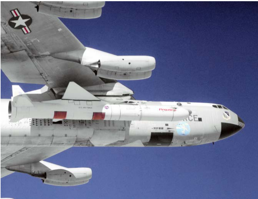
This is the first Orbital Sciences Corporation Pegasus winged booster on a captive-carry flight under NASA's Boeing NB-52 Stratofortress mother ship, November 1989. (NASA)
