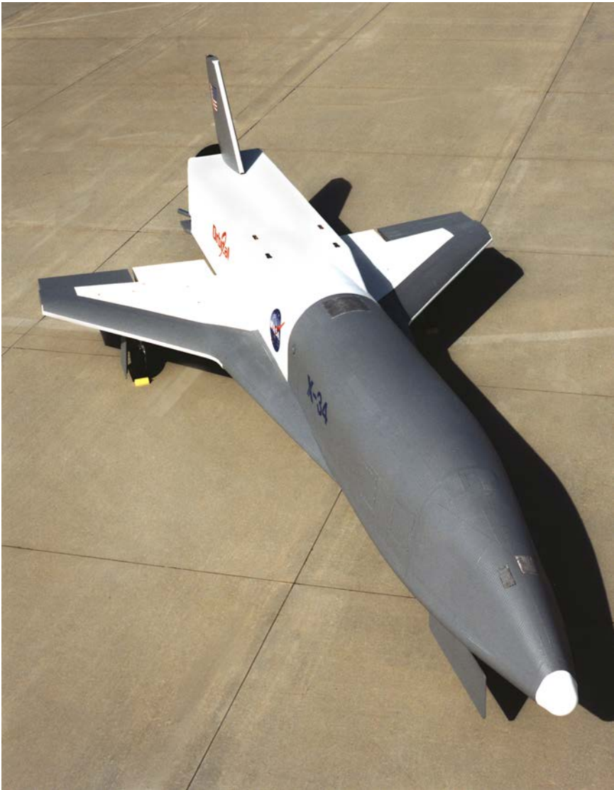
The X-34 A-1 Structural Test Article on Rogers Dry Lake, April 16, 1999, showing its distinctive high-finesse-ratio fuselage and double-delta planform. (NASA)
