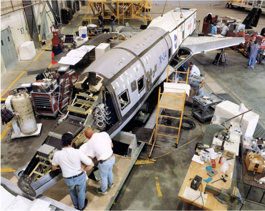
NASA and Orbital X-34 test personnel at Dryden are modifying the X-34 A-1 for air launch, October 1999. (NASA)
