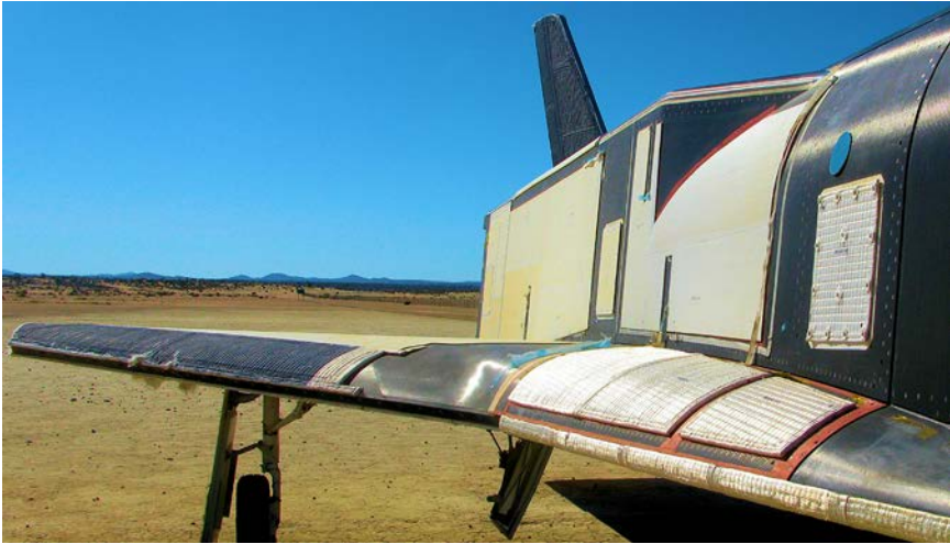
The X-34 A-2 shown with its double-delta wing, the graphite/epoxy composite skin structure, and portions of the thermal protection system blanket overlay, March 17, 2010. (RPH)
