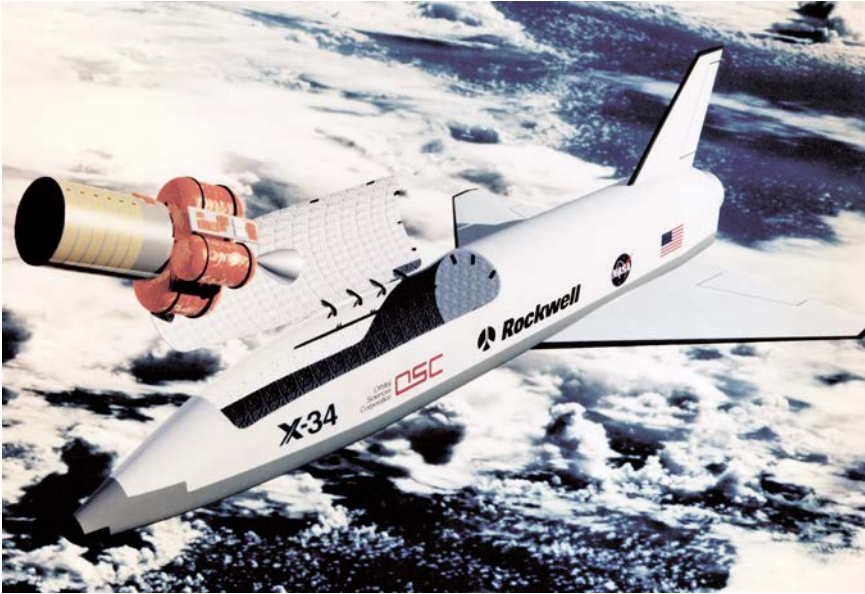
An October 1995 depiction of an X-34 RLV shows it releasing a satellite payload, which will then boost into orbit. (OSC)
