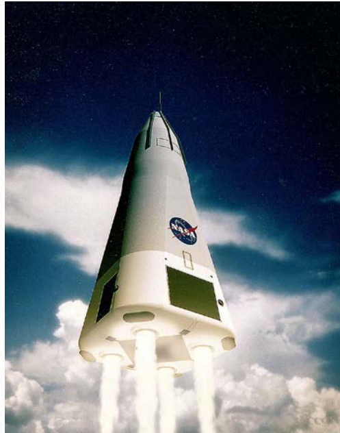
DC-X proponents hoped it would lead to a future single-stage-to-orbit reusable launch system, the VTOL McDonnell Douglas DC-XA, shown in this conceptual depiction. (NASA)
