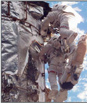
Large radiation-induced cracks in the outer layer of multilayer insulation after years of space exposure (Townsend et al., 1999).
