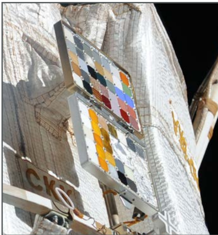
Figure 20. Russian Replaceable Cassette-Container on the Russian Service Module.
