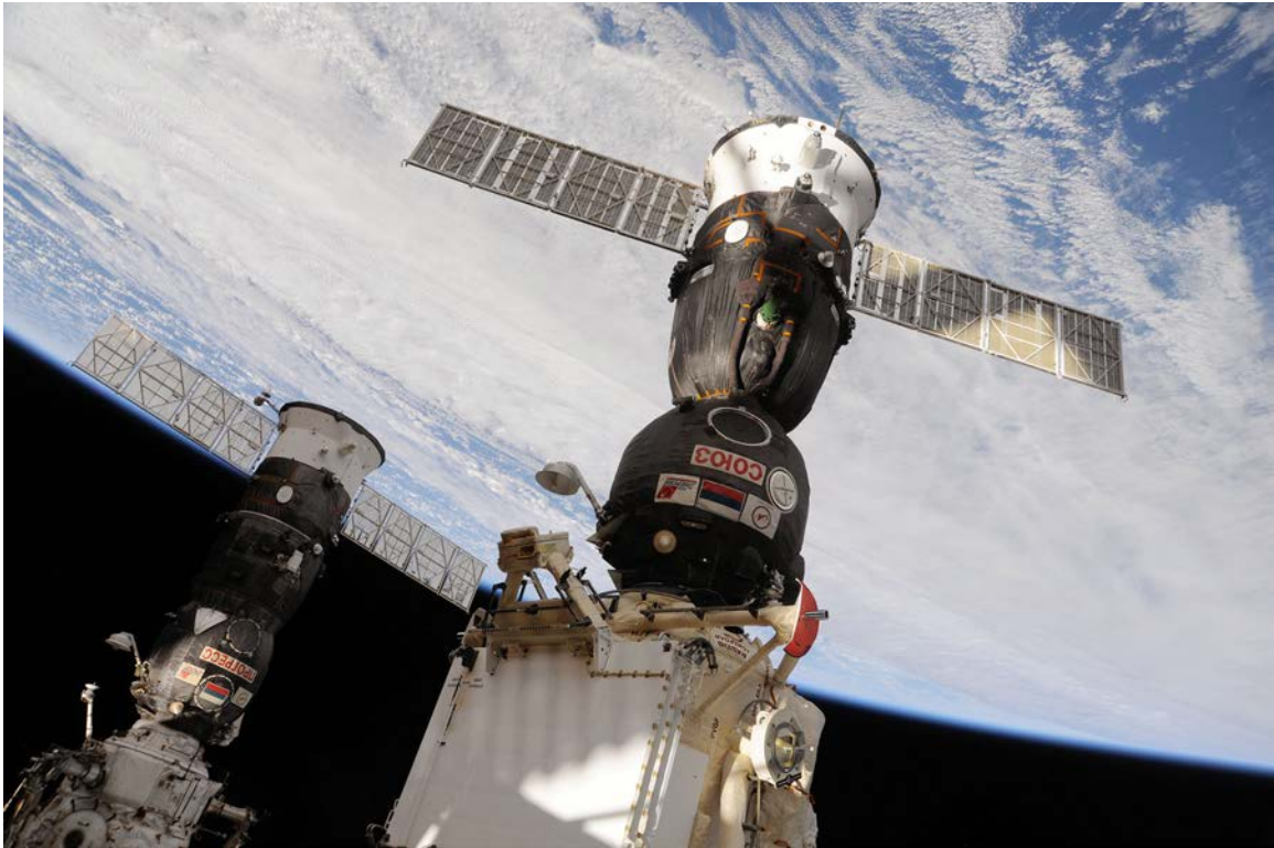
FIGURE 10. Rassvet. The Soyuz TMA-19 spacecraft (foreground), docked to the Rassvet Mini-Research Module 1 (MRM1), and Progress 37 resupply vehicle, docked to the Pirs Docking Compartment, are featured in this image photographed by an Expedition 24 crewmember on the ISS. (NASA ISS024-E-007122)
