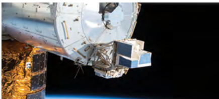
On the left is a picture of the HDEV system attached to the European Space Agency Columbus External Payload Facility. On the right is a snapshot of footage from the HDEV, capturing a view of Tropical Storm Leslie. The storm struck the Iberian Peninsula and the East Coast of the United States in September and October 2018.
