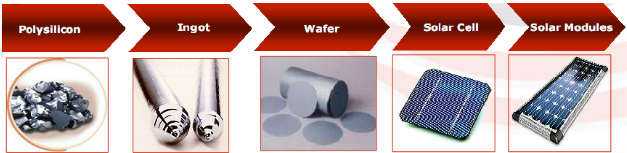
Figure 2.1-9. Flow Diagram of the Crystalline Silicon PV Value Chain.
