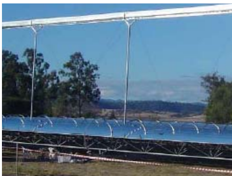
Figure 2.2-4. Linear Fresnel System
